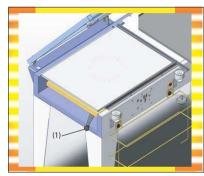
(1) Easy adjustment of product delivery tray height Optional manually operated tray raising and lowering feature: lever (1)
